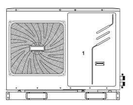
**Door 1**: Gives access to the compressor compartment, to the hydraulic compartment and to the electrical parts
