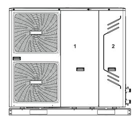
**Door 1**: Gives access to the compressor compartment and electrical parts
