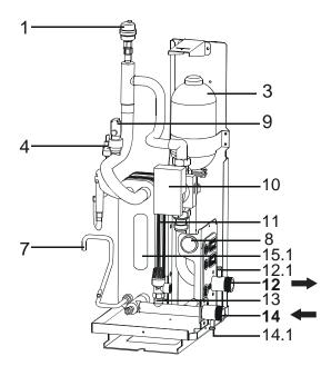
**1.Air purge valve.** Remaining air in the water circuit will be automatically removed via the air purge valve.
