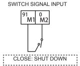
**NOTE:** when this digital input is closed the unit and the remote controller are locked. To unlock theme is necessary to open the digital input.
