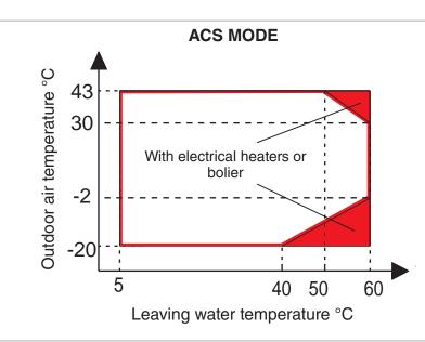
NOTE FOR DHW MODE: leaving water temperature is the temperature of the water produced by the unit and not the DHW temperature available to the user; the DHW temperature is in fact a function of this parameter and of the coil surface of the DHW boiler.
