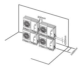
2. In case of installing multiple units (2 units or more) in lateral connection per row.
